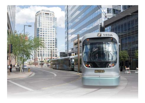
Another type of railway is light rail transit (LRT). It also operates using electricity. The power is usually provided by an overhead electrical line. LRTs often run on tracks in the middle of a street or beside a street. They may have one car or several cars and carry up to several hundred people per trip. LRT is seen by many as a clean, modern form of mass transit.
